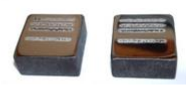
Figure 5. Samples for preliminary experiment with electro-spark coating, 20 x 20 x 10 mm
