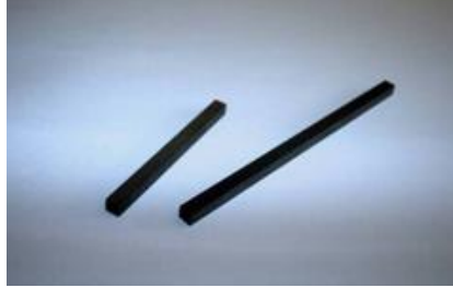
Figure 4. Shape of the electrodes, 3x3x80 mm
